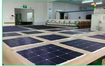
Solar panel lamination
