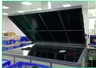
EL testing for foldable solar panel
